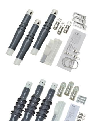
TE's Raychem CSTI/O cold shrink terminations are made from a high performance, liquid silicone material which is specially formulated for excellent tracking and split resistance. The extra-long silicone stress cone is integrated within the termination which ensures correct positioning. Moisture sealing at the lug is integrated into the termination body, eliminating the need for additional sealing tapes.
