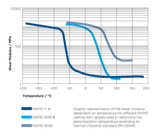
RAPID casting resins are available in different grades according to the functional requirements of the particular application: From materials featuring rubber elasticity and low glass transition temperature for sensitive electronics to tough and rigid materials for mechanical protection or classic insulation technology.
