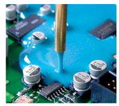
RAPID polyurethane casting resins can easily be handled with ordinary two-component dispensing devices.
