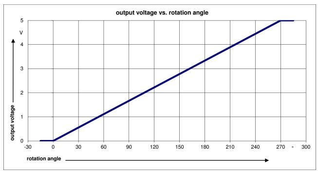
Figure 4: Output voltage vs. rotation angle
