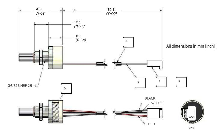
Figure 1: Dimension of the ED-22 (side view)
