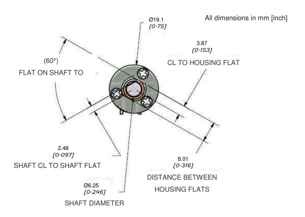
Figure 3: Dimension of the ED-22 (front view)
