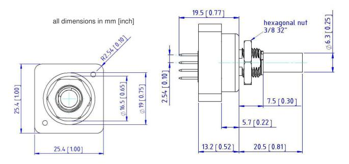
Figure 1: Dimensions of the ED-19-SB-XXXX-X-X (top and side view)
