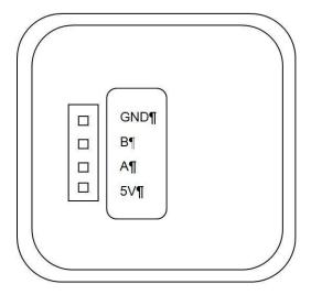
Figure 3: Pinning of the ED-19-XX-XXXX-X-X (bottom view)
