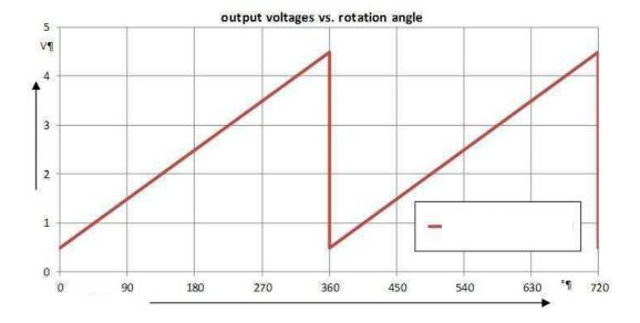
Figure 4: Output voltage vs. rotation
