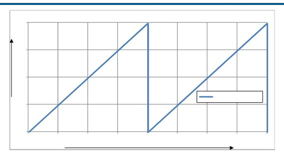
Figure 5: Output current vs. rotation angle
