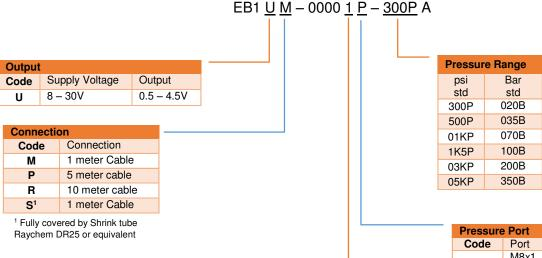
The **psi** range models are only supplied with imperial thread design. The **bar** range models are only supplied with metric thread design
