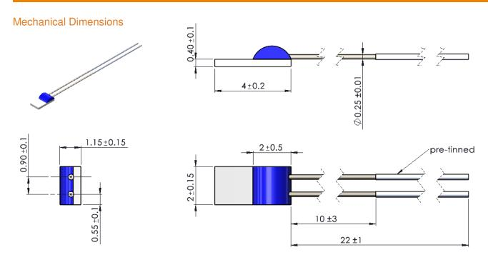
Figure 1: Mechanical dimensions of Platinum Temperature Sensor
