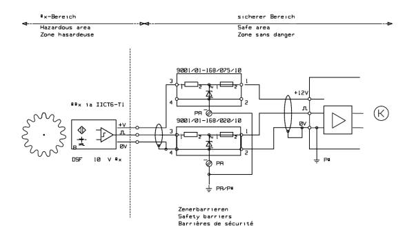
Connection diagrams (refer to dimensional drawing for exact type): • Sensor types DSF xx10.00 AHV Ex-atex:
