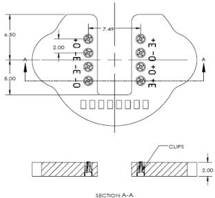
Note: Recommended use the PCB with clips press-fit or solder to the pin of sensor, for details of PCB and Clips, please consult TE.
