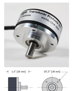
The CS15 is Celesco's compact industry standard size 15, servo-mount incremental encoder. With a low profile of less than an inch in height and a diameter of only 1.5 inches, the economically priced CS15 is perfect for both the OEM and single-piece user alike. Precision ball bearings support a durable stainless steel shaft for reliable, long life operation.
