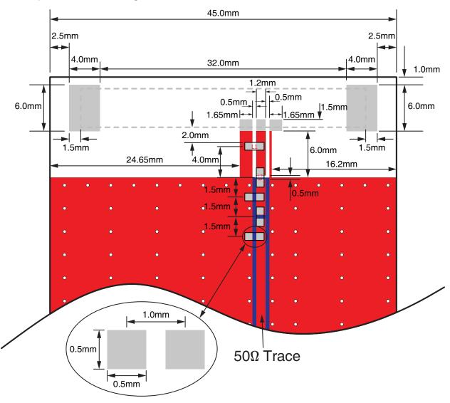
Component values are determined through testing. Contact Linx for more information on matching network assistance.
