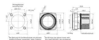
Main Dimensions Receptacle \*for max. wire cross-section pay attention to the cross-section of used contacts
