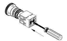
1-2. Separate contact block housing from actuator housing. Wires can be terminated to the terminals of the contact block housing.
