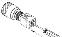
1-2. Separate contact block housing from actuator housing. Wires can be terminated to the terminals of the contact block housing.
