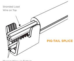
Magnet Wires on Bottom
