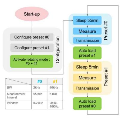
With the example, every 1 hour will result of having 2 measurements: one with a high frequency band and another (5min later) with a low bandwidth but with a higher resolution.
