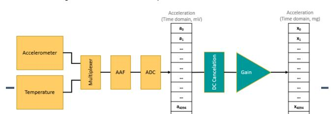
When the system requests a data measurement, the sensor acquires 4096 data points at the required bandwidth. The information below shows the relationship between sampling frequency, bandwidth, and acquisition duration (warm-up and processing times are not included):
