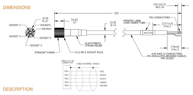
Piezo resistive plug and play accelerometer cable assembly featuring #12-48, 5-socket plug. Standard cable length is 120 inches. Mates with accelerometer model 4807A.
