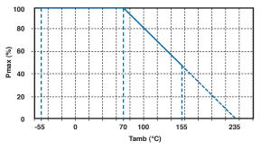
Maximum dissipation (Pmax) in percentage of rated power as a function of ambient temperature (Tamb)
