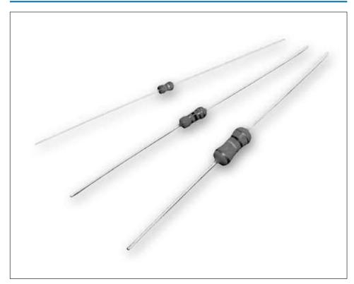
The RR Series is manufactured by depositing a homogeneous film of metal alloy onto a high-grade ceramic body. After a helical groove has been cut in the resistive layer, tinned connecting wires of electrolytic copper are welded to the end-caps. The resistors are coated with a red, non-flammable lacquer, which provides electrical, mechanical and climatic protection. The coating is resistant to all cleaning solvents in accordance with MIL-STD-202, method 215 and IEC 60068-2-45.
