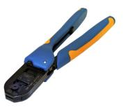
to confirm that any specific combination of hand tool, terminal, and wire can be crimped. This requires considering the force required to achieve optimum compression over the entire range of terminals and wire applicable to a given tool. The wire crimp jaws will be calibrated to bottom at the maximum crimp force requirement for each specific tool.
