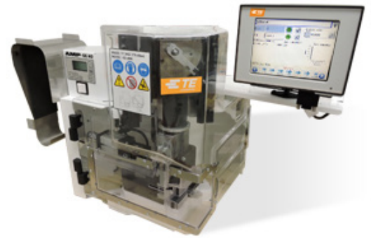
Pig-tail Splice Model
