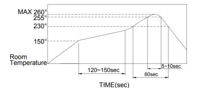
■ The condition noted above is the temperature of the copper foil on the surface of the PCB. There are cases where the temperature of the board greatly differs from the surface of the switch. Do not allow the surface temperature of the switch to exceed 260°C.
