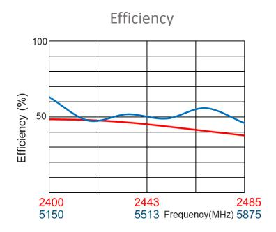
Data measured in free space and under plastic device enclosure
