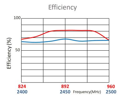
Data measured in free space and on plastic device enclosure
