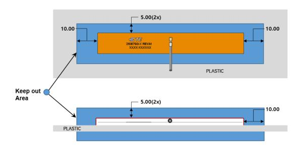
NOTES: 1. Antenna designed to be mounted on plastic cover.
