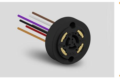
ANSI C136.41 COMPLIANT DIMMING RECEPTACLE PROVIDES AN ELECTRICAL AND MECHANICAL INTERCONNECTION BETWEEN AN ANSI C136.41-2013 COMPLIANT CONTROL AND LUMINAIRE.
