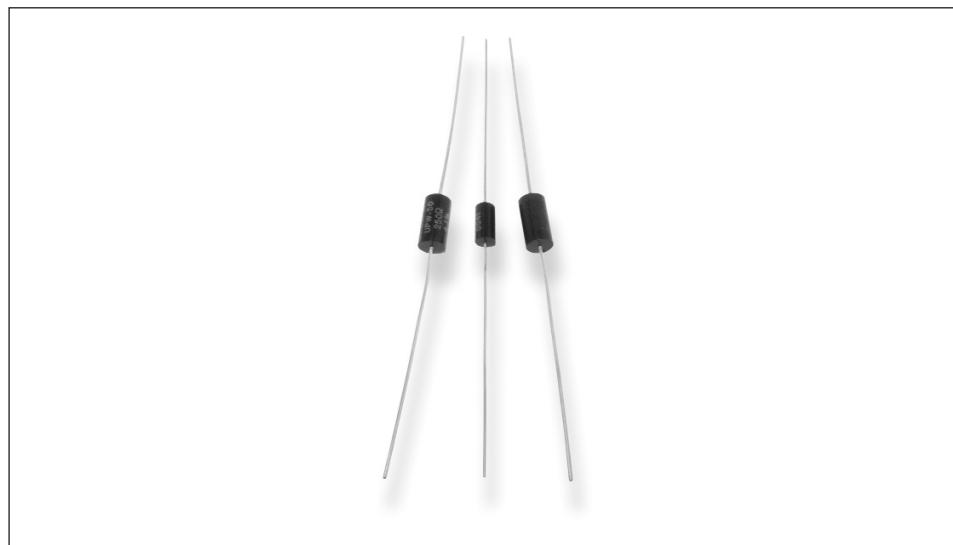
The resistive element is wire wound onto a moulded high temperature plastic bobbin with a central former. The direction of winding is reversed part way through the winding, giving very low values of inductance. These Neohm resistors use bobbin assemblies with flattened lead ends, providing high resistance to pull, vibration and torsional forces during handling, assembly and life.
