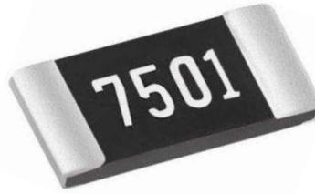
TE are pleased to introduce the new 3504 series. This is a high stability Thin Film Chip Power resistor range offering very high power / size ratio – 6W in 2512 size. The 3504 series offers TCR at  $\pm 50\text{ppm}/^\circ\text{C}$  and resistance tolerance at  $\pm 1\%$  as standard. Resistance values are within the IEC 63 E96 and E24 value grids. The 3504 resistors have accurate and uniform physical dimensions to facilitate automatic placement methods.
