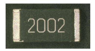
TE Connectivity is pleased to introduce this thick film high power device, sister to our popular 3522 series, suitable for auto placement in volume and for most applications. Supplied as standard on 7 inch Reels of 1000 pieces per reel.
