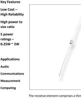
The resistive element comprises a thin film of carbon, deposited onto a high thermal conductivity ceramic core. Metal end caps are force fitted to the element prior to spiralling to value. Tinned copper lead wires are welded to the end caps and the components are then coated. One coat of phenolic resin is followed by three coats of epoxy resin. All resistors are tested for value and tolerance.
