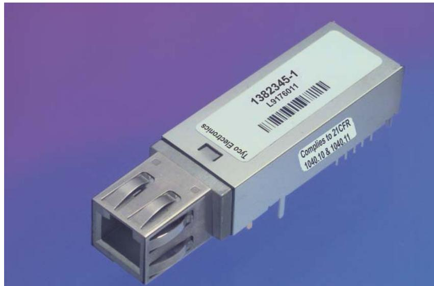
Tyco Electronics' ESCON/SBCON SFF MT-RJ Transceiver 1382345-1 is an LED based 1300 nm fiberoptic transceiver module intended for use in ESCON and SBCON applications. The transceiver sends and receives pre-encoded data over a pair of 62.5  $\mu\text{m}$  or 50  $\mu\text{m}$  core multimode optical fibers. The module, which operates from a single +3.3V power supply, contains separate transmitter and receiver sections with PECL and LVPECL compatible data interfaces.
