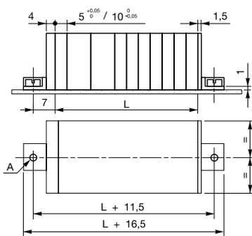
$$L = (N \text{ блоков} \times 5.05) + (N \text{ блоков} \times 10)$$
