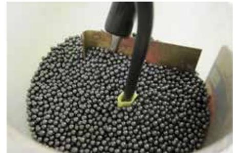
Figure 6 - Dielectric Strength Test - PLASTI-GRIP Terminal
