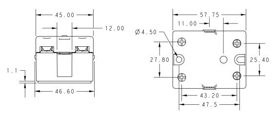
\*Overall height dimensions includes with clear cover Dimensions in mm
