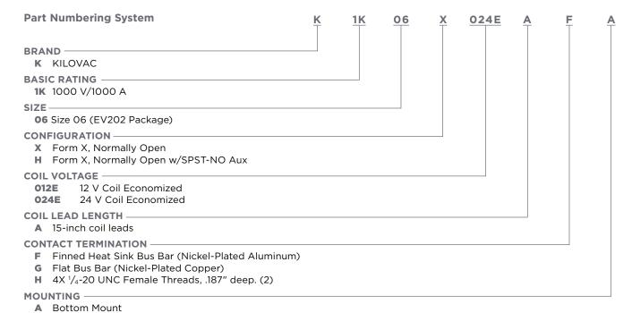
(2) User furnished bus bar must be equivalent to 4X 4/0 conductor. Torque to 45-55 in-lbs. per connection (5.1 - 6.2 NM)
