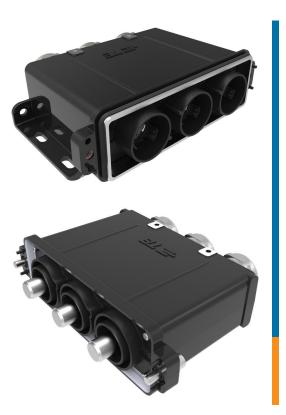
Rugged power connectors for all mission critical power applications on rolling stock, meeting EN 50467 including requirements for fire and smoke compliance per EN 45545-2. Allowing multiple combinations with just ten variants this connector series saves weight, space and contains more electrical capacity up to 650 amps, 4000 volt.
