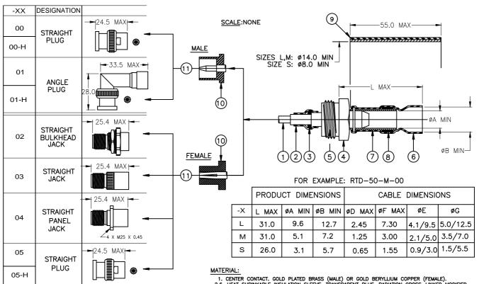
⊕ -H PARTS HAVE HEX NUT COUPLING WITH LOCK WIRE HOLES.
