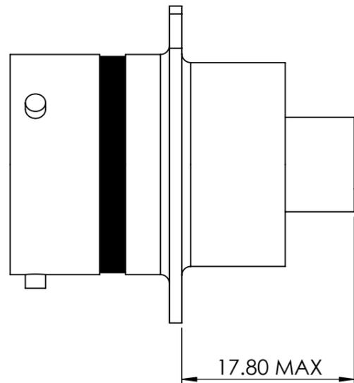
VIEW SHOWING PROTRUSION OF CRIMP CONTACT WHEN INSTALLED
