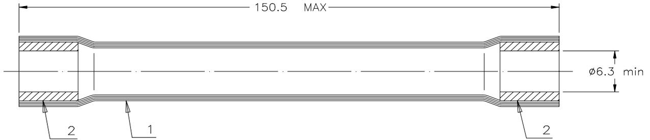
1) BLACK OUTER HEAT-SHRINKABLE TUBING WITH SEALING INSERTS
