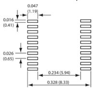
The MT Series encoders and decoders are implemented in an industry standard 20-pin Shrink Small Outline Package (20-SSOP)
