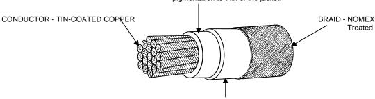
JACKET - RADIATION-CROSSLINKED, MODIFIED ETFE
