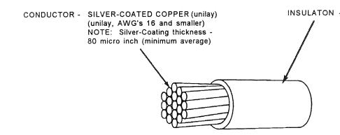
INSULATON - RADIATION-CROSSLINKED, MODIFIED ETFE
