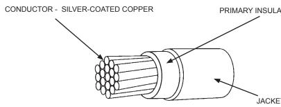
PRIMARY INSULATION - RADIATION-CROSSLINKED. MODIFIED ETFE Primary insulation shall be of a contrasting pigmentation to that of the jacket.
