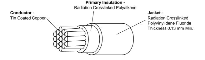
Part Wire Conductor Conductor **FINISHED WIRE** Size Stranding Diameter Diameter Maximum Description Maximum (AWG) No./AWG (mm)Resistance (mm.) Weight @20°C (kg/km) Min. Max. Min. Nom. Max.  $(\Omega/km)$ 44CD0811-8-\* 8 133/29 4.01 4.39 2.30 5.28 5.44 5.59 93.5
