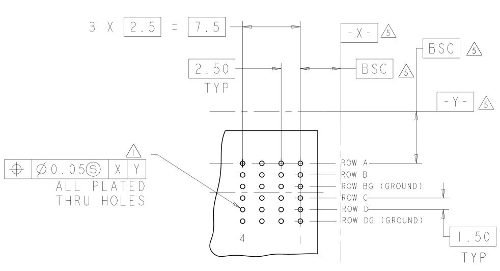
▲ 0.70mm ±0.025 DRILLED HOLE 0.025 MIN - 0.050 MAX COPPER PLATING THICKNESS 0.0002 - 0.0005 ORGANIC SOLDERABILITY PRESERVATIVE (OSP) 0.62 REF NOMINAL FINISHED HOLE SIZE DIMS AND TOLERANCES APPLY TO TOP 1.40 OF PCB THICKNESS. A MATERIAL : CONTACT FINISH: MATING PRODUC GR-121 ENVIRO COMPLIA TIN-LE
