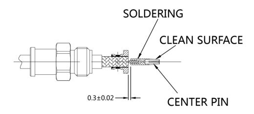
4.A. Insert the cable into the main body until it reaches the end face of the insulator on the cable contact with the insulator step inside the main body and cannot be pushed until.
