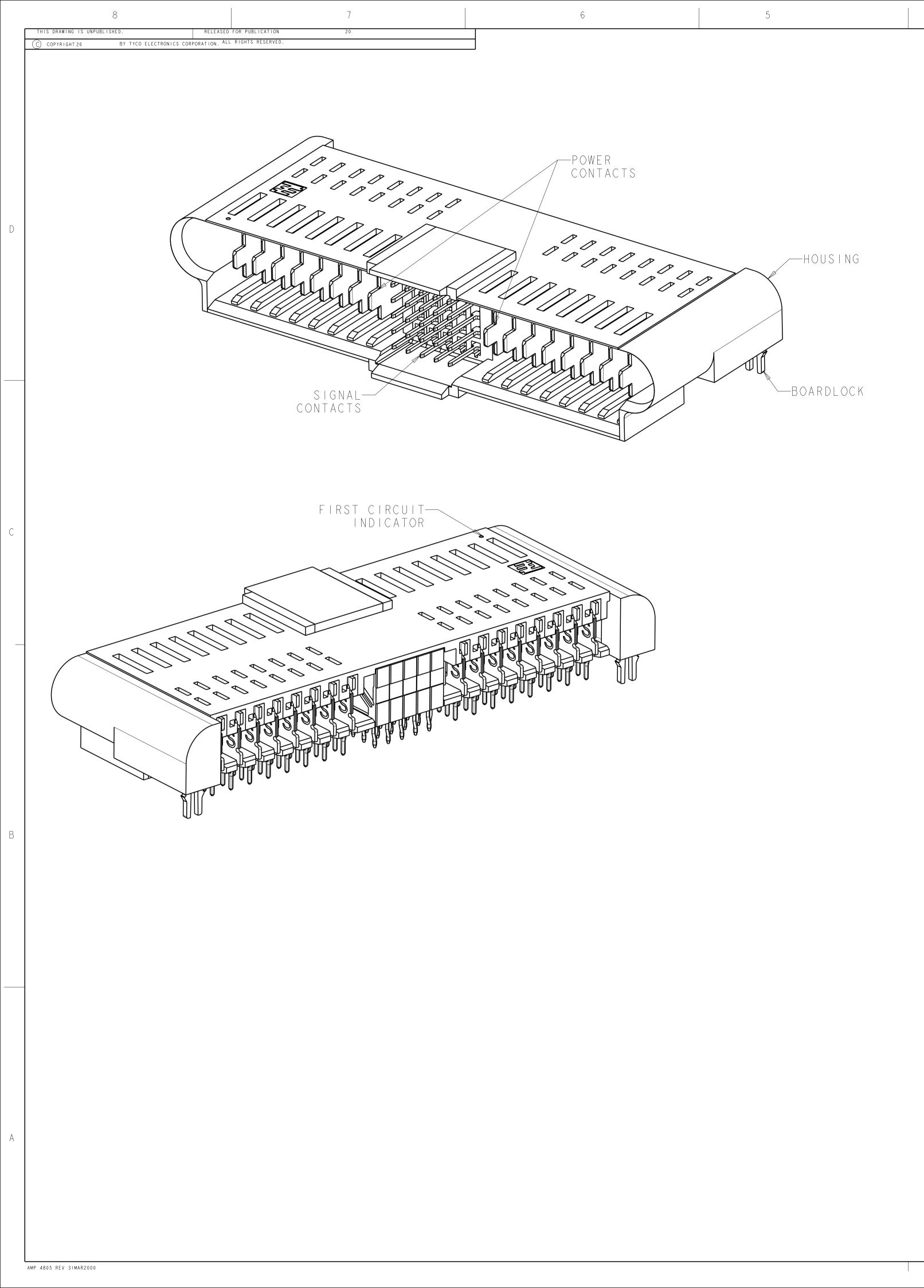
I. HOUSING: GLASS FILLED LIQUID CRYSTAL POLYMER, COLOR: BLACK, UL 94 V-O RATED SIGNAL CONTACT: PHOSPHOR BRONZE SIGNAL OVERMOLD: GLASS FILLED POLYESTER POWER CONTACT: COPPER ALLOY BOARD LOCK: PHOSPHOR BRONZE
