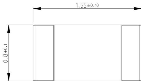
FOR FURTHER INFORMATION SEE DATA SHEET FOR RP73 SERIES-SMD HIGH POWER PRECISION RESISTORS
