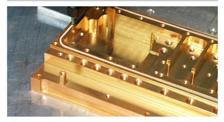
Form in place is a conductive elastomer, being conductive silicone in liquid form for depositing direct to enclosure hardware.
