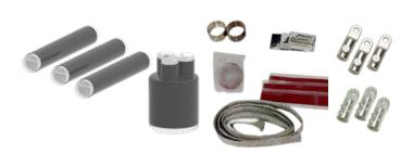
TE's Raychem Cold Shrink Terminations CSTI/O are made from a high performance, liquid silicone material which is specially formulated for excellent tracking and split resistance. The extra-long silicone stress cone is integrated within the termination which ensures correct positioning. As an option, moisture sealing at the lug can be integrated into the termination body, eliminating the need for additional sealing tapes.
