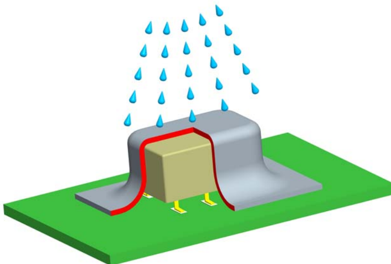
Fig. 11: Coating of relays on PCB's
