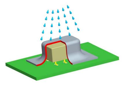
Fig. 4: Coating of relays on PCB's
