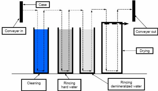
Fig. 3: Cleaning of PCB's. It is most essential to keep the temperature level during cleaning, rincing and drying constant. The temperature shall not deviate by more than  $\pm 10^{\circ}$ C.
